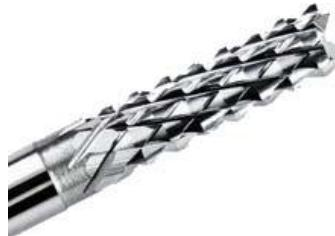
They're great for finishing cuts, but their material removing capacity is limited relative to other kinds of bits. Since they're gentle on the material, they are often used with composites, PC board material, and other layered materials.
